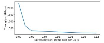
Fig. 7: Negative correlation between throughput and network traffic cost
