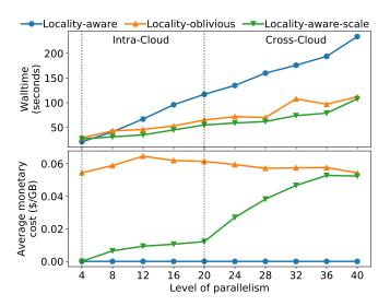
Fig. 8: Comparison of end-to-end runtime and network traffic cost with different scheduling strategies as job concurrency increases
