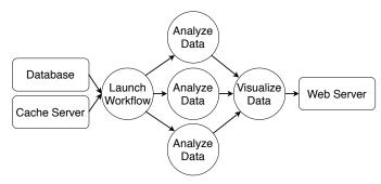
Fig. 3: An example of appliance: the workflow launcher waits on the database and cache server up and running before starting the workflow; the workflow spawns a number of parallel data analysis jobs that generates output data; the data visualization job visualizes the output data in observation that all the job analysis jobs are done; finally, the web server is started to render the visual after the data visualization job succeeds.
